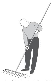
When the pole is fully extended, insert it into the hole on top of the base ensuring it locates in the bottom hole.
