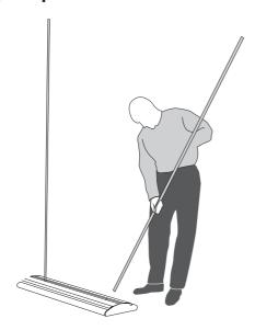
The Premier 1250 Wing has two poles that are made up and inserted in the same way, as shown above
