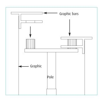
Attach the 'T' bar to the top of the pole and gently extend each graphic panel so that the 'T' bar slots into the hole on each graphic bar.
