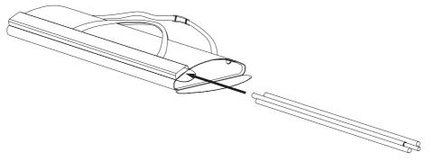
Place the pole in the special pocket on the outside of the bag.
