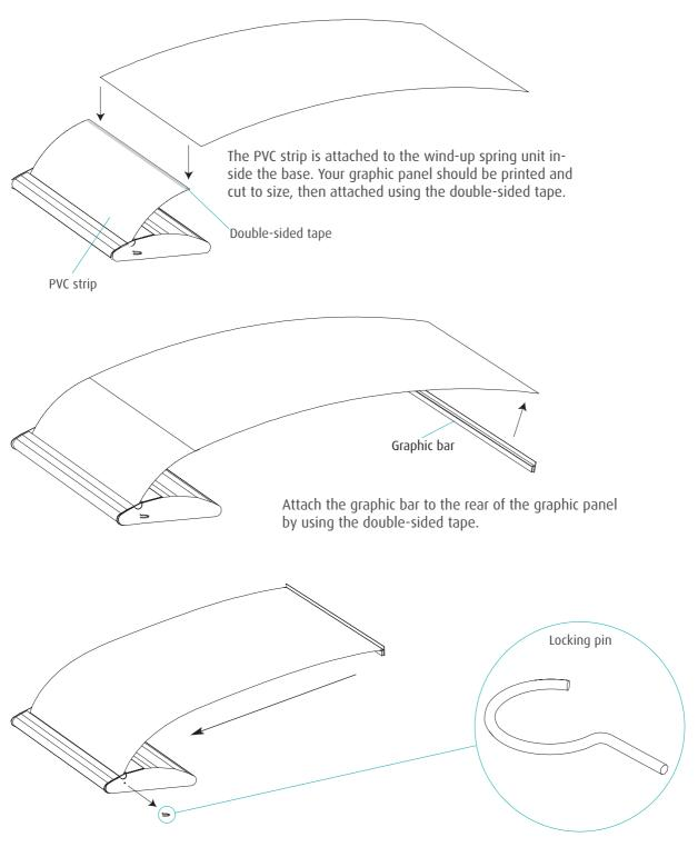
Whilst securely holding the graphic panel, remove the locking pin to release the spring and carefully guide the graphic panel into the base.
