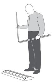
Place the base on the floor and unfold the pole until the three component slots together to form a rigid pole.
