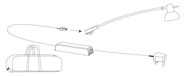
The 75 watt low voltage light kit comes with a transformer, a 3m cable, a light bracket, bulb and a bag. The 75 watt main voltage light comes with a 3m cable, alight bracket, bulb and a bag.
