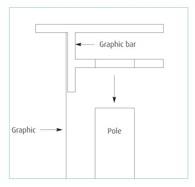
On the underside of the graphic bar that is attached to the top of the graphic panel you will see a hole. Standing behind the Premier Wing, extend the graphic panel until you can locate this hole with the top of the panel.
