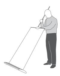
Standing behind the banner, from the side holes of the base pull the graphic bar up and extend it towards the top of the pole (s).
