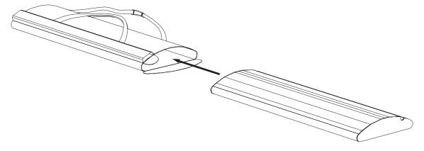
With the graphic panel within the base, place the base inside the bag
