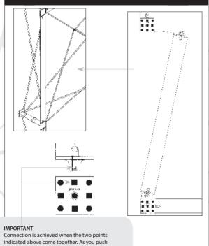
indicated above come together. As you push the mag bar into the 4-Way junction, you will hear a click, which indicates a secure connection
